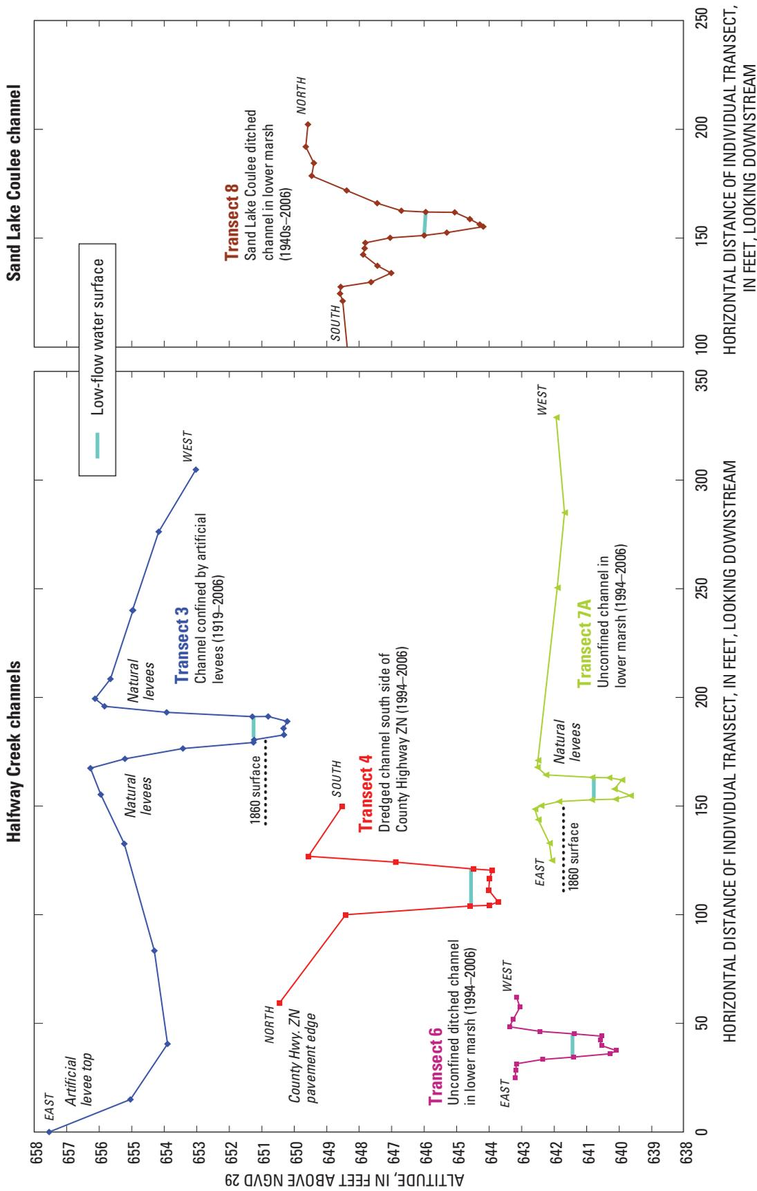
Figure 15. Channel cross sections of Halfway Creek and Sand Lake Coulee, Wis., 2006. Transects are not horizontally related. Locations of transects are shown on figure 1B.
