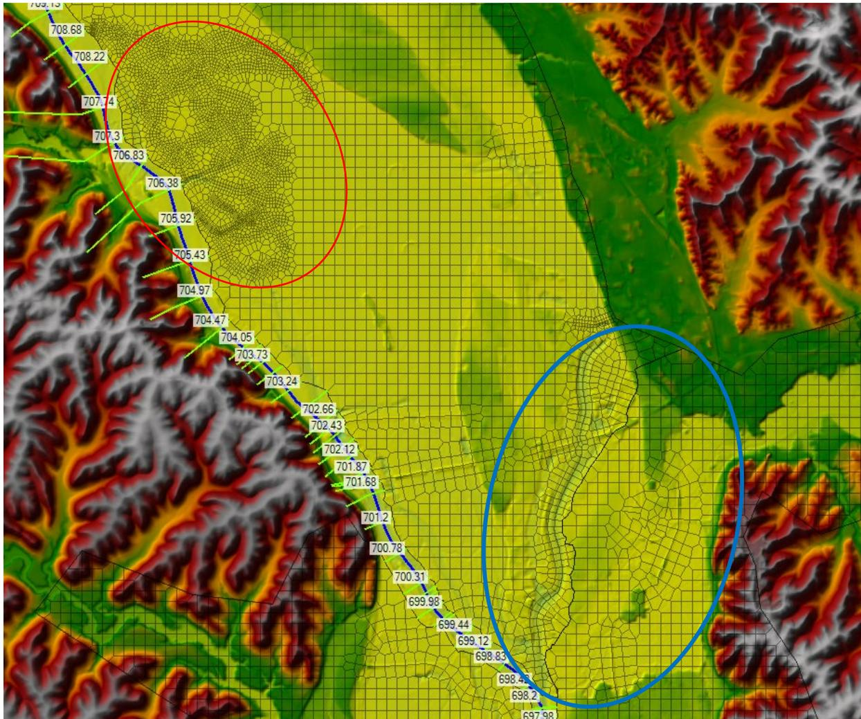
Figure 3: Adjusted Geometry (project area in red and modifications to the Black River in blue)
