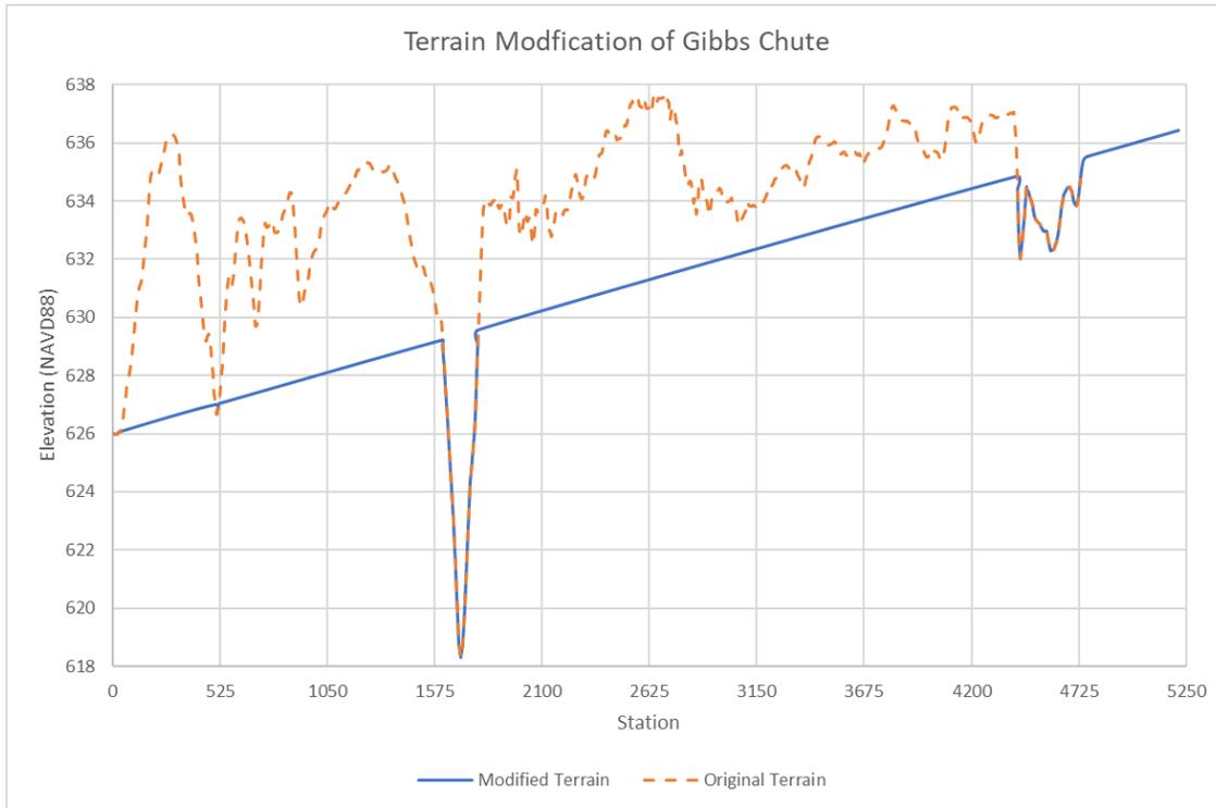
Figure 33: Modified Vs. Original Terrain of Gibbs Chute
